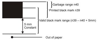
For every step the paper is feed, the black mark sensor is sampled to detect garbage, black marks or out of paper.
